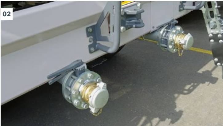
02 Connections for water and emulsion are easily accessible.
