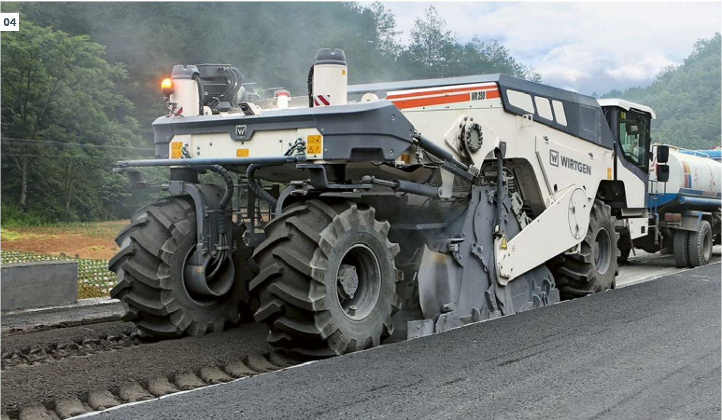
01 - 04 In cold recycling, damaged asphalt layer are granulated, mixed with binding agents, processed, compacted, and repaved.
