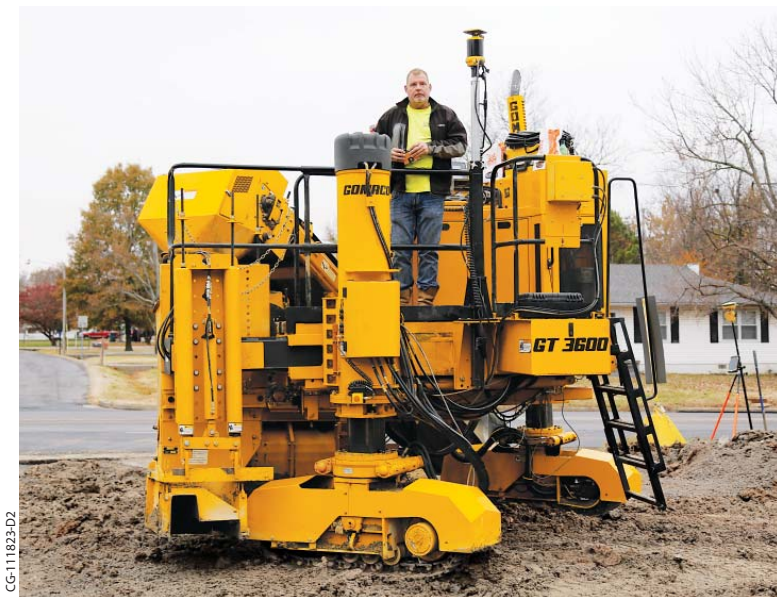
The Xtreme GT-3600's tracks can rotate farther than ever before. The rotary-sensored slew drives allow the tracks to rotate 90 degrees and more for quick side travel and job-site mobility.
