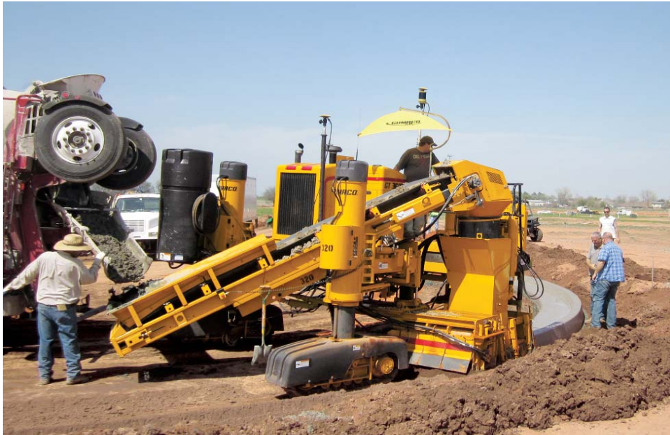
This GT-3600 uses the simultaneous trim/pour process for maximum concrete utilization.
