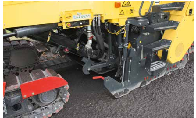
Optimum sealing of the inner conveyor belt increases reliability and reduces dust pollution.
