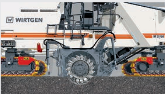
3 | Cold milling machine is lowered slowly while retaining its parallel alignment
