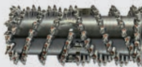
Standard milling drum Milling width: 2,000 mm Milling depth: 0-330 mm Tool spacing: 15 mm
