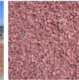
Recycled brick chippings
