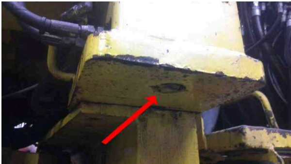
Lifting cylinder right side is leaking
