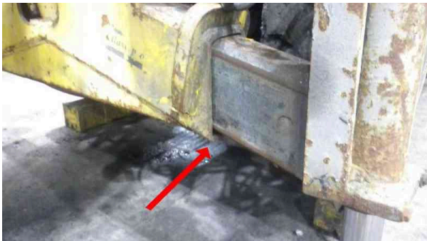
Outrigger need to be rebuilt,loose
