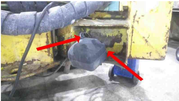
Rear right light broken
