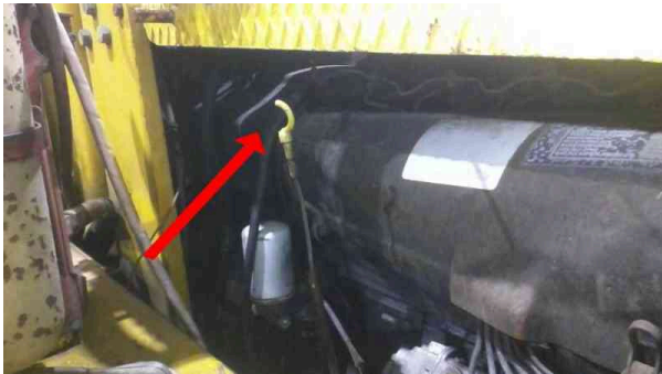
Engine dipstick broken, Engine #F5L912W S/N:8740752
