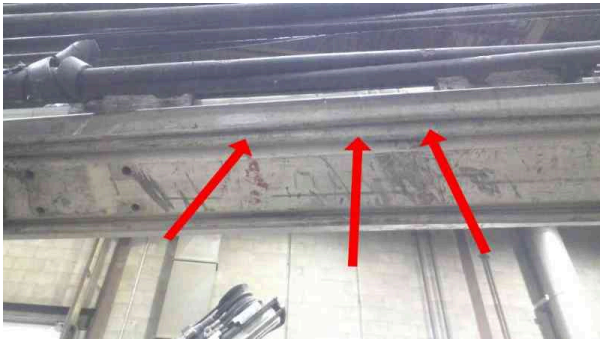
Slide cover take off and dirt underneath
