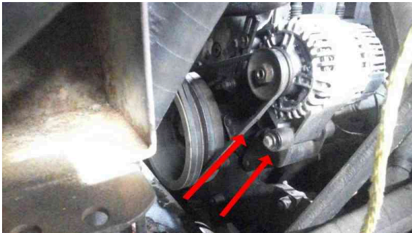
Alternator and alternator belt have to be replace
