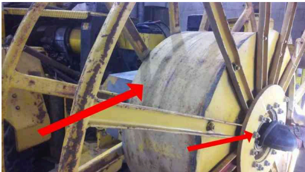
Cable is not secure in the cable reel and cable is missing
