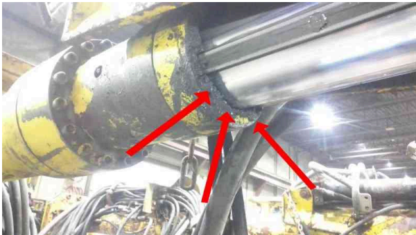
Boom extension cylinder loose in the tefflons and leak internally
