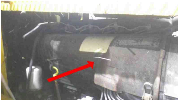
E-stop not working, shut off cable on the engine broken
